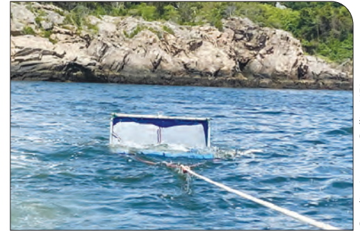
A neuston net towed behind a research team's boat
