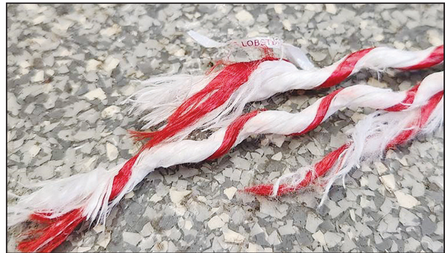
Tested 1700 lb. candy cane rope with MASS LOBSTER tracer ribbon
