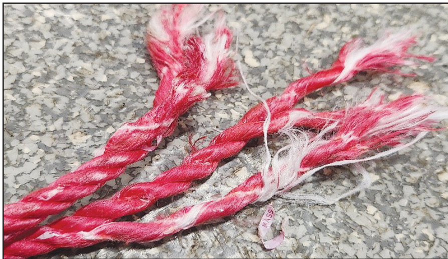
Tested 1700 lb. red rope with MASS LOBSTER tracer ribbon
