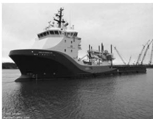
Shelia Bordelon Flag: US Clearance Method: ROV with boulder grab and pre-lay mattress installation IMO: 9670638
