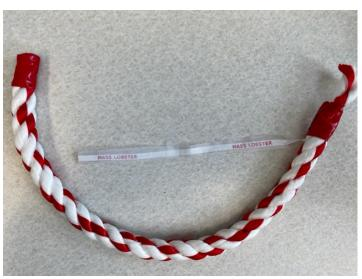
tested by NOAA Gear Specialist, Rob Martin, which were found to be within the acceptable breaking strength allowance.
