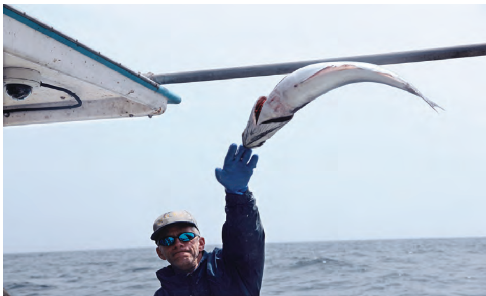
A mounted camera (top left) records catches and discards under an electronic monitoring pilot program. – The Nature Conservancy photo
